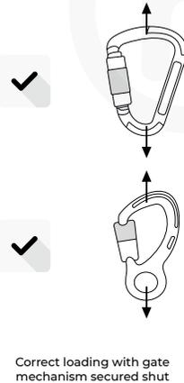
Correct loading with gate mechanism secured shut
