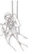
• Heavy weight with high speed in a long distance descent= quick release of gravitational potential energy, the high temperature generated on descender could damage the rope or lower control performance.
