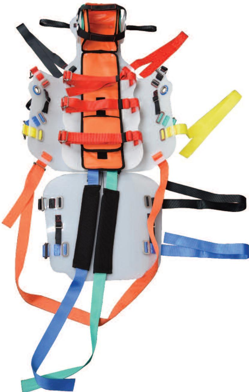
The Slix50 has been designed for difficult confined spaces. The articulated skirt at the bottom of the stretcher can be removed. When in place it provides protection for the upper legs and allows a degree of bending for tight spaces. Hauling points are located on the top and sides of the stretcher for maneuverability. The side hauling points will hold the stretcher in a semi-horizontal position.
