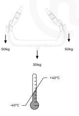
Product Details WSOI is a work seat by At Height. It has a moulded stainless steel frame covered with comfortable padding for prolonged use in suspension. Two side dee rings are fitted, each with a WLL of SOkg. There is an additional webbing loop on the underside for easy carrying and it has a WLL of 30kg.
